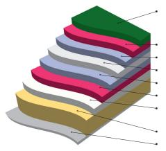
High Performance coating applied to the weather side of the steel sheet (Juniper Green or Slate Grey) Primer Galv Steel substrate Galv Primer Light Grey polyester coating on reverse side of steel sheet 40mm Polyisocyanurate (PIR) insulation core 50micron Internal Liner Aluminium Foil
