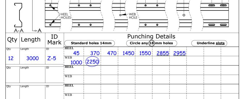
The purpose of this leaflet is to demonstrate the use of the Order Form for Purlins & Rails. Above is a section of the Purlin & Rails Order Form. The information filled in relates to the purlin drawn underneath which has been transcribed for explanatory purposes. The terms "HEEL" and "WEB" relate to the cross section and are labelled below. Holes are defined by their location and the distance from the start of the member. 18mm holes are circled and slots underlined.
